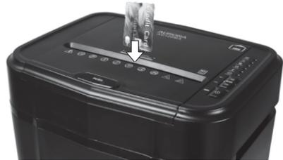
Insert one credit card at a time into the middle of the feed slot.
