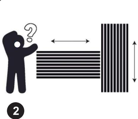
Decide the direction in which the acoustic panels will be mounted. Panels can be shortened from the back using a skill saw or fine-toothed blade.
