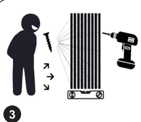
Install the panels with black screws through the polyester into the wall or the ceiling. Screws are strategically positioned left to right at the bottom, middle and top of each panel.
