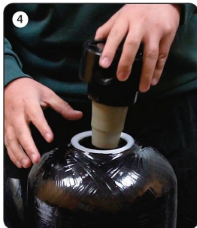
Insert the centre tube firmly into the constructed head then install into the tank
