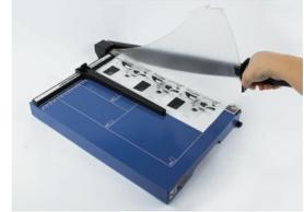
3. Firmly push down on the spring loaded bottom lip of safety shield to hold the paper firmly when cutting.
