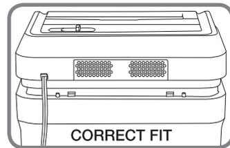
**5** Make sure the shredder head is correctly mounted.
