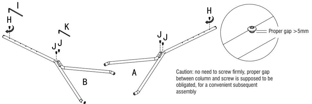
Caution: no need to screw firmly, proper gap between column and screw is supposed to be obligated, for a convenient subsequent assembly
