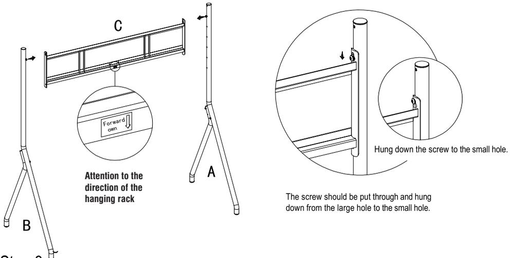
The screw should be put through and hung down from the large hole to the small hole.
