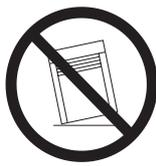
The weight of the shredder is concentrated on the upper part of the machine, making it top heavy. Please place the machine upright on a flat level surface to avoid it falling-over and causing damage or injury.
