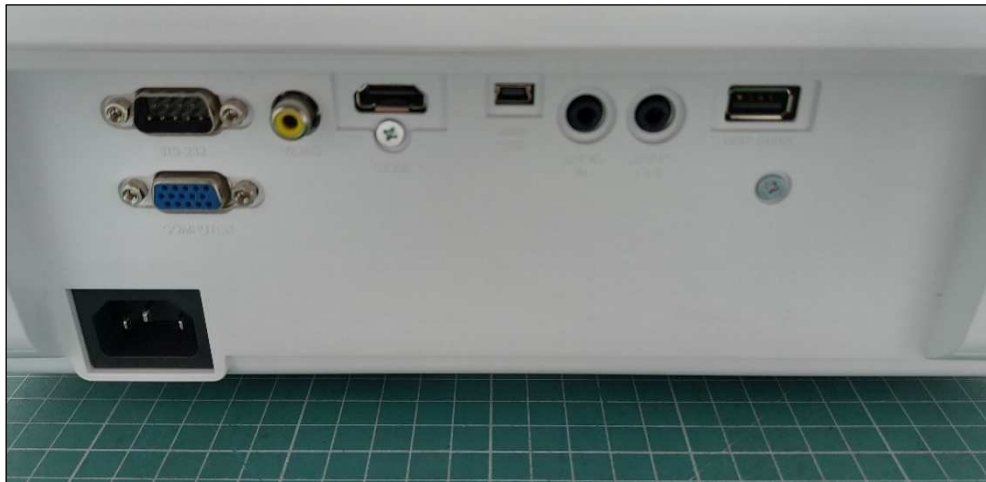
Figure 5: Enclosure appliance coupler and IO ports
