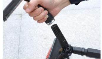
③ Insert the glass scraper onto the three-way gimbal to fix it.
