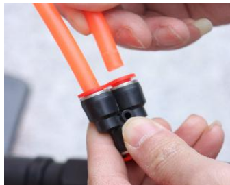
① Assembling the manifold
